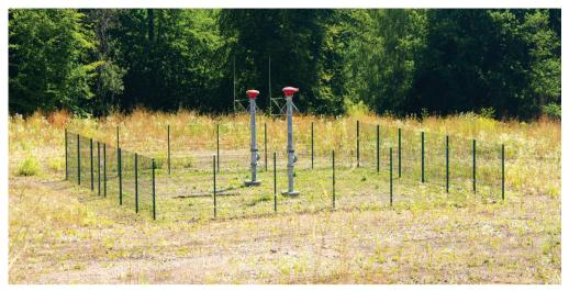
Fig. 3. An installation for degassing liquidated coal workings – the only element marking the former location of mining shaft *Lauterbach* on the border between Saarland and the Moselle district (photo by P. Langer, 2015)
