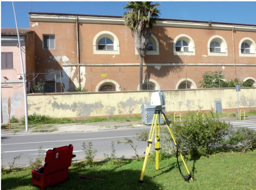
III. 6. The photo presents the capturing phase of the architectural survey using Laser Scanner 3D Leica C10 all-in-one
