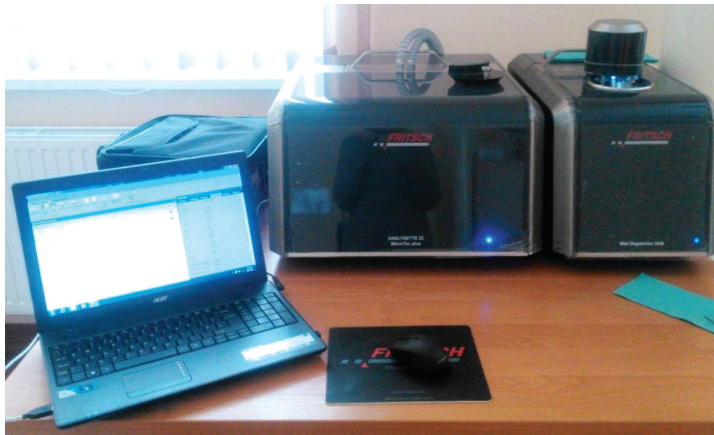
Fig. 2. Laser particle-size meter Analysette 22 MicroTec Plus applied in the research
