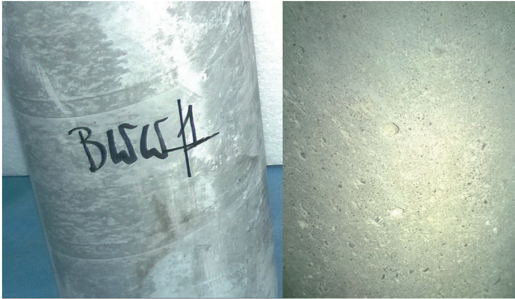
Fig. 1. The concrete surface before (left) and after sandblasting process (right) in the case of HPC
