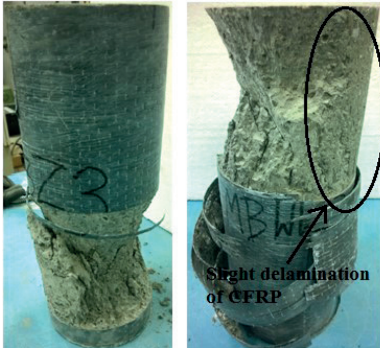
Fig. 4. Failure modes of NCC-CFRP (left) and HPCC-CFRP (right)
