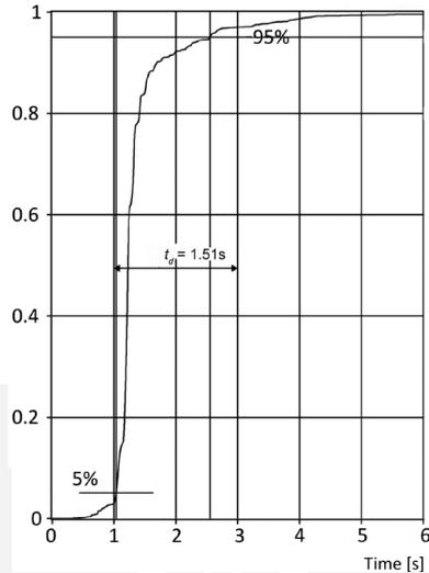
Fig. 3. Normalised Arias intensity versus time (Husid plot) for the Panewnicka Street station horizontal records of April 18<sup>th</sup> 2015 rockburst (Fig. 2)
