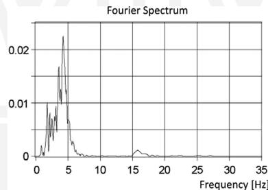
Fig. 4. Fourier spectrum of the acceleration component the Panewnicka Street station horizontal 'y' record of April 18<sup>th</sup> 2015 rockburst
