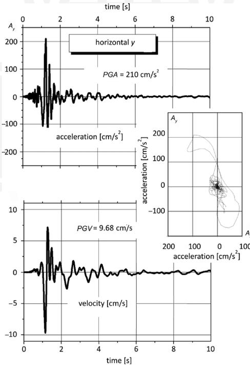
Fig. 2. Accelerations and velocities of the April 18<sup>th</sup> 2015 rockburst horizontal record as measured along the ‘y’ axis of the Panewnicka Street recording station (inset: image of simultaneous spatial, horizontal x and y accelerations)
