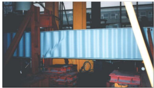
Fig. 8. Failure mode for the SIN type profile according to [10]
