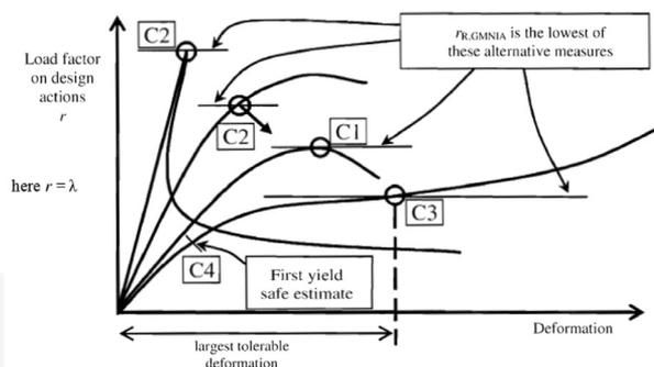
Fig. 13. Definition of buckling resistance from global GMNIA analysis [6]
