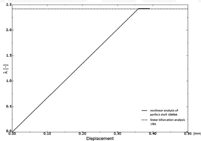
Fig. 5. Path of equilibrium for the analysed shell
