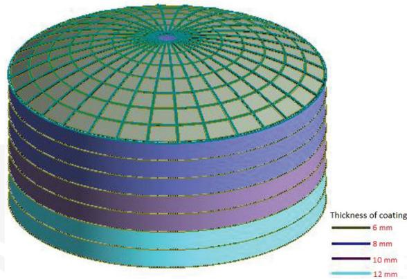
Fig. 4. Model of the tank in Autodesk Robot Structural Analysis 2015. Linear bifurcation analysis
