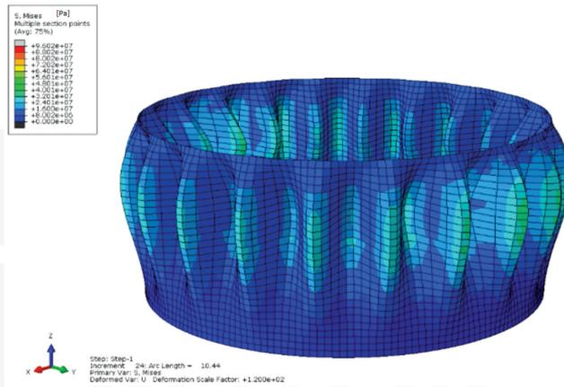
Fig. 6. Deformation of the shell with the map of stress before reaching limit point
