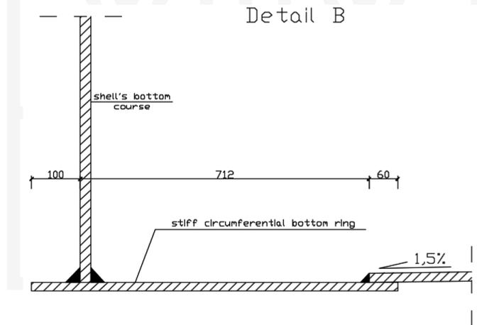
Fig. 1b) Detail B: fixed connection shell bottom
