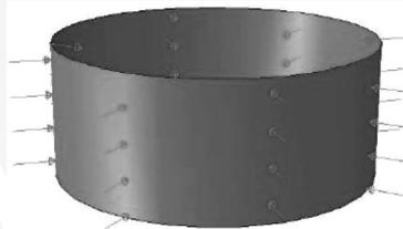
Fig. 2. Pressure normal to the shell surface
