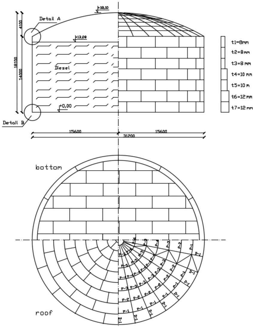
Fig. 1. Geometry of the tank
