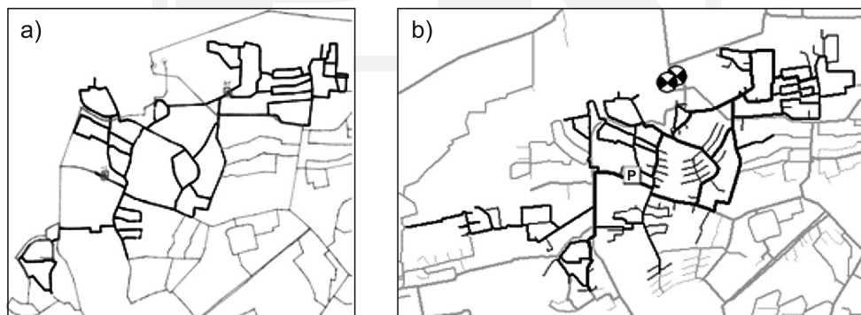
Fig. 1. Water supply system-black contour line marks pipes served by the Silver Eagle pressure tank: a) in 1993, b) in 2010
