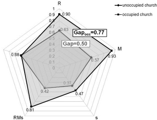
Fig. 9. Assessment of acoustic properties of the unoccupied and occupied the St. Elizabeth of Hungary Church using the modified index method with the Gap and Gap<sub>occ</sub> indices
