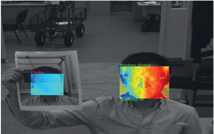
Fig. 9: Three-dimensional machine vision system for smart railway stations, discriminating between the 3D face of a person (right) and a 2D photograph of their face (left), where green is among the colors used to visually represent the face during surface gradient reconstruction. Photograph © Centre for Machine Vision, Bristol Robotics Laboratory, University of the West of England, Bristol, UK. Used with kind permission
