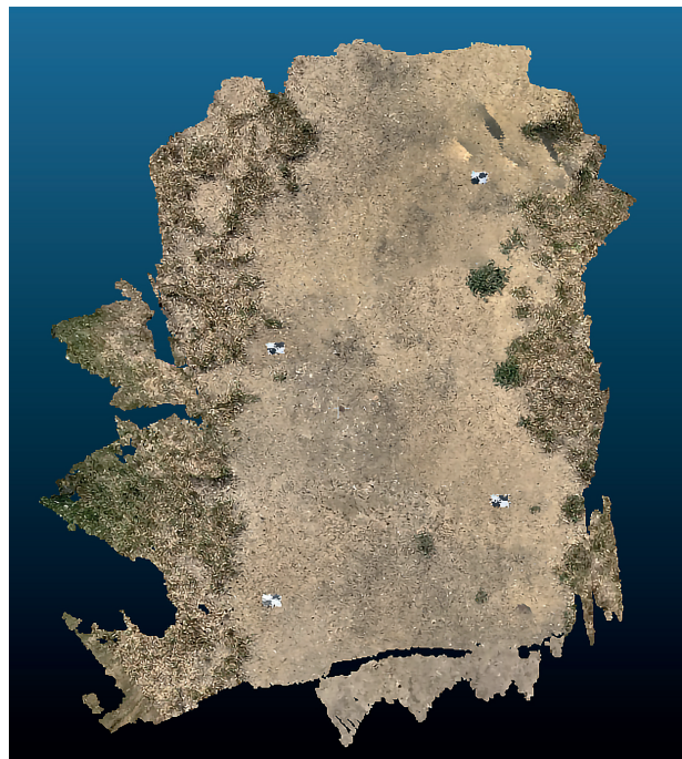
Fig. 2. The point cloud of the test object with four target markers in CloudCompare
