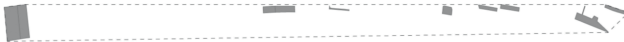
Fig. 2. Example of a convex boundary – dashed line, for registration parcels (dark grey polygons) belonging to one registration unit
