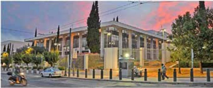
**Image 12.** US Embassy in Athens - zonal security in the form of static road barriers, high fencing, a permanent guard booth for law enforcement and road patrol.
