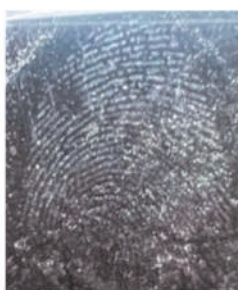
Fig. 2. Fingerprint showing good visibility on glass surface kept for 168 h
