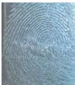
Fig. 7. Fingerprint showing very good visibility on tempered glass surface kept for 30 min
