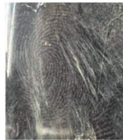
Fig. 9. Fingerprint showing poor visibility on steel surface kept for 240 h
