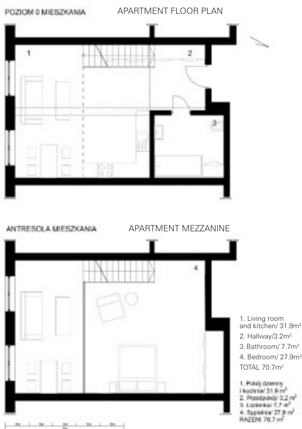
III. 10. Floor plans of a two-room apartment (with mezzanine, type 1) at the Lofty De Girarda investment venture (author's own collation based on sources from Żyrardów Starosty archives)
