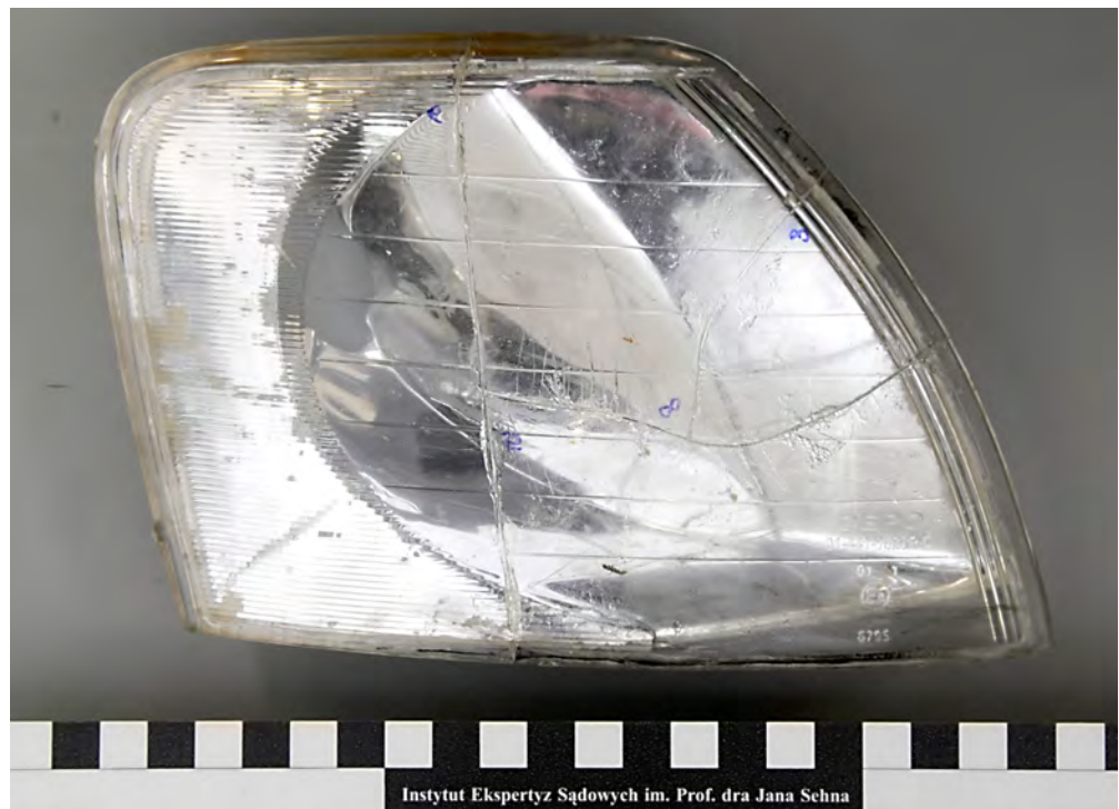
Fig. 5. Transparent plastic fragments and silver-coloured plastic fragments before reconstruction. Source: Institute of Forensic Research in Kraków.
