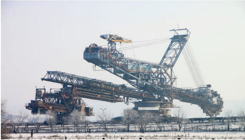
Fig. 6. Bucket wheel excavator
