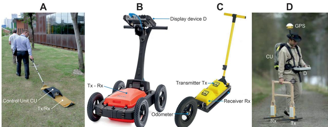
**Fig. 1.** Examples of typical configurations of the GPR systems produced by different geophysical companies – systems with: A) monostatic antenna ([www.radsys.lv](http://www.radsys.lv)); B) nonseparated bistatic antennae ([www.geophysical.com](http://www.geophysical.com)); C) separated shielded antennae ([www.sensoft.ca](http://www.sensoft.ca)); D) separated unshielded antennae ([www.guidelinegeo.com](http://www.guidelinegeo.com))
