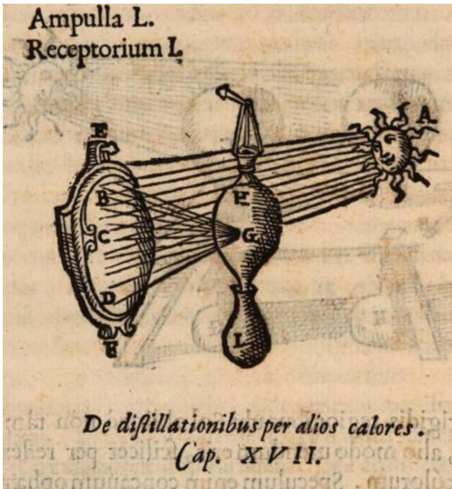
Fig. 14. Distillation in a vessel warmed up using a concave mirror (source: G. della Porta, De distillatione lib. IX [...], Romae 1608, p. 30)
