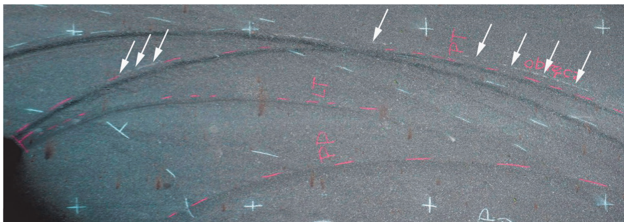
Figure 12. Marks left by the slipped tire (dark) and those left by the steel rim indicated with arrows.
