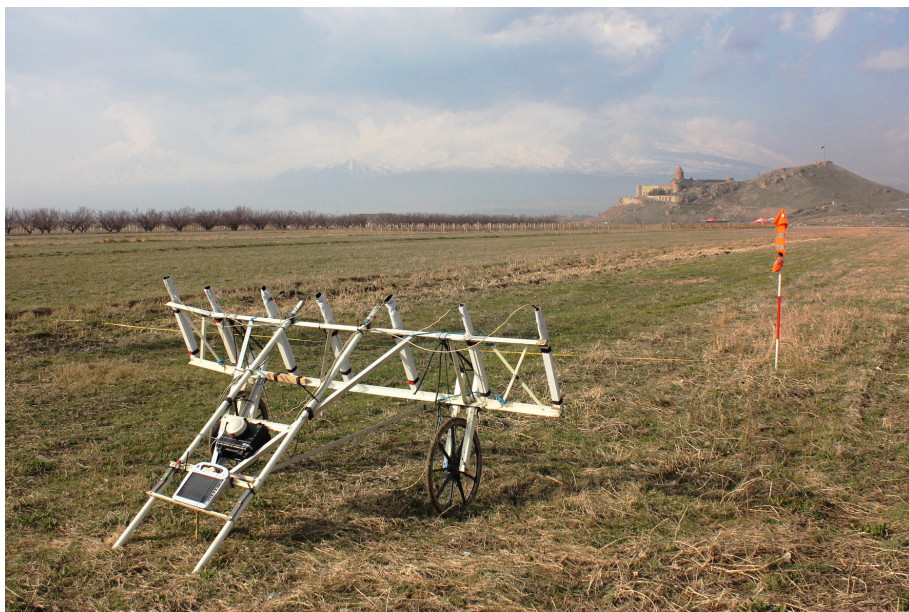
Fig. 3. LEA MAX system carrying seven gradiometer probes (© Armenian-German Artaxata Project)
