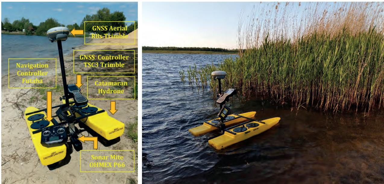
**Fig. 4.** Measurement set applied in profiling the bottom of the Piaseczno water body (vessel Hydron Seeffloor, echosonar OHMEX – converter P66, positioning of sonar: GNSS receiver R8s Trimble + controller TSC3 Trimble)
