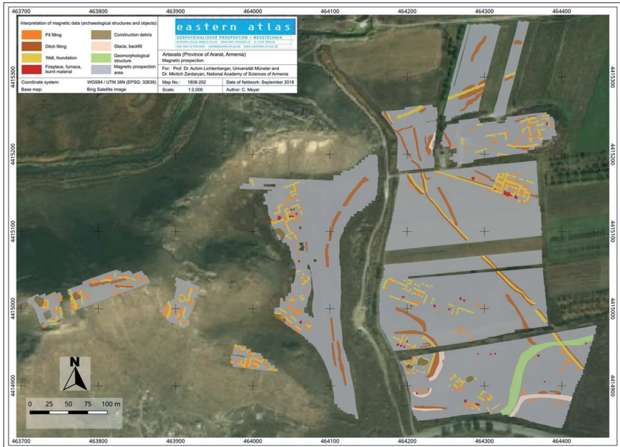
Fig. 8. Interpretation of the magnetic prospecting in Artaxata 2018 (by Eastern Atlas)
