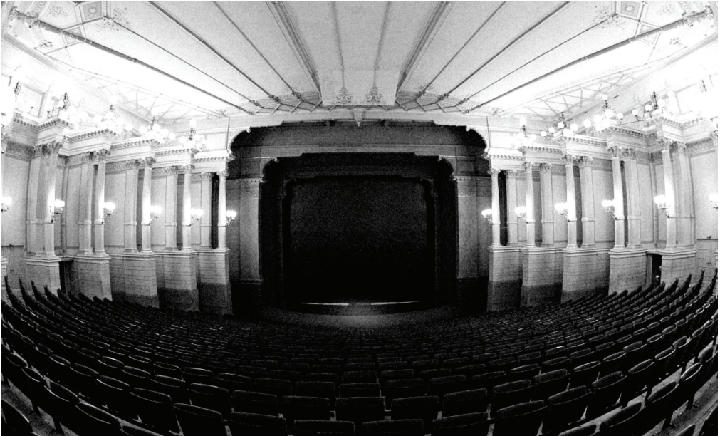
Fig. 4. Bayreuth, Margravian Opera House. The auditorium formed as horseshoe was a baroque standard, the visibility from the lodges was limited (photo by P. Obracaj) Bayreuth, Festspielhaus. The fan-shaped auditorium provides a full view of the scene (fisheye, photo by P. Obracaj)
