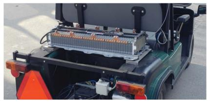
Fig. 3. Rear part of the tested vehicle with NiMH battery
