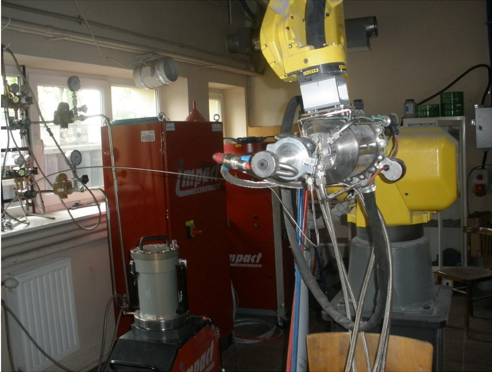
Fig. 2. Impact Innovation 5/8 cold spray system
