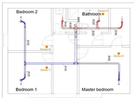
Fig. 3. First floor – sensor layout
