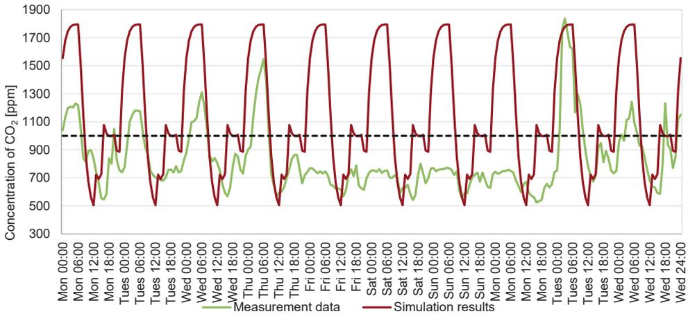
Fig. 7. Carbon dioxide concentration – simulation with the minimal ventilation rate and closed door to the walk-in wardrobe; maximum recommended level of 1,000 ppm marked by the dashed line
