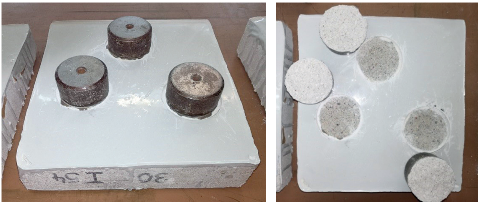
Fig. 10. View of the sample before (left) and after (right) detachment of the steel discs
