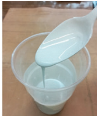
Fig. 6. Epoxy coating mixed with glass powder
