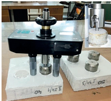
Fig. 8. A view of the test bench for pull-off testing
