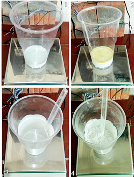
Fig. 5. The stages of preparation of the resin coating (1 – resin, 2 – addition of hardener, 3 – mixing of components, 4 – addition of glass powder)
