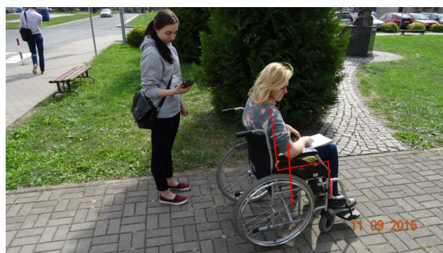
Fig. 3. The position of the person's body during the tests: a) passive drive – position A; b) active drive – position B
