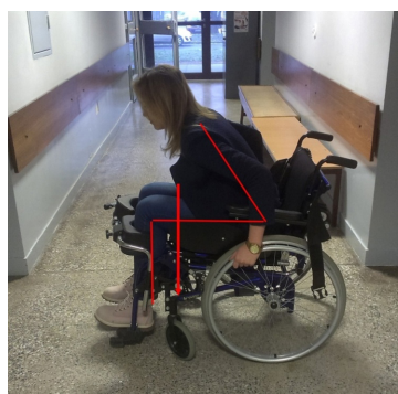
Fig. 3. The position of the person's body during the tests: a) passive drive – position A; b) active drive – position B
