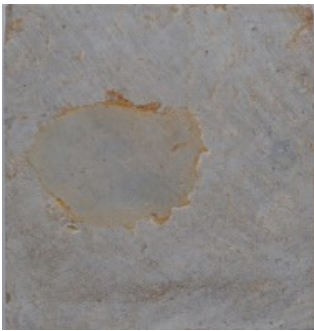
Fig. 8. Examples of sample cut surface views with visible gaps filled with a yellow-rust colored substance [10]
