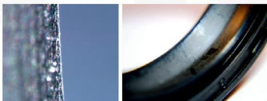
Fig. 8. The effects of the sealing ring wear
