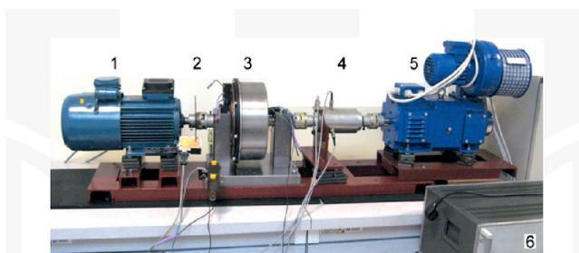
Fig. 7. View of the test bench with the installed dual clutch: 1 – electric motor, 2 – dual clutch, 3 – torque meter, 4 – electric brake, 5 – high voltage power supply
