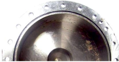
Fig. 9. Corrosion spots inside the dual clutch housing
