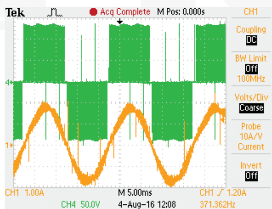
Fig. 9. Phase-to-phase voltage (CH4) and phase current (CH1) waveform before sinusoidal filter from inverter side
