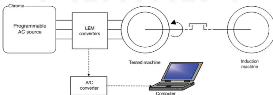
Fig. 2. Diagram of the measurement system
