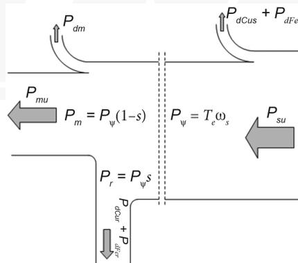
$P_{su}$  – stator power;  $P_{\psi}$  – rotating field power;  $T_e$  – electromagnetic torque;  $\omega_s$  – rotating field pulsation;
