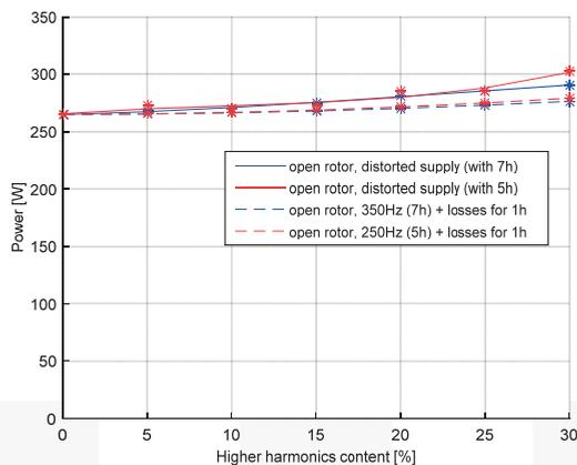
Fig. 12. Study of the additivity of losses. Iron losses, comparison
