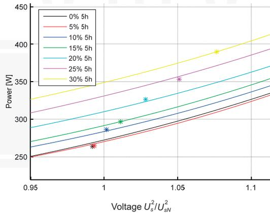
Fig. 8. Idle run losses, for voltage with various amount of 5 harmonic added (with winding and mechanical losses subtracted) shorted rotor, zoomed section
