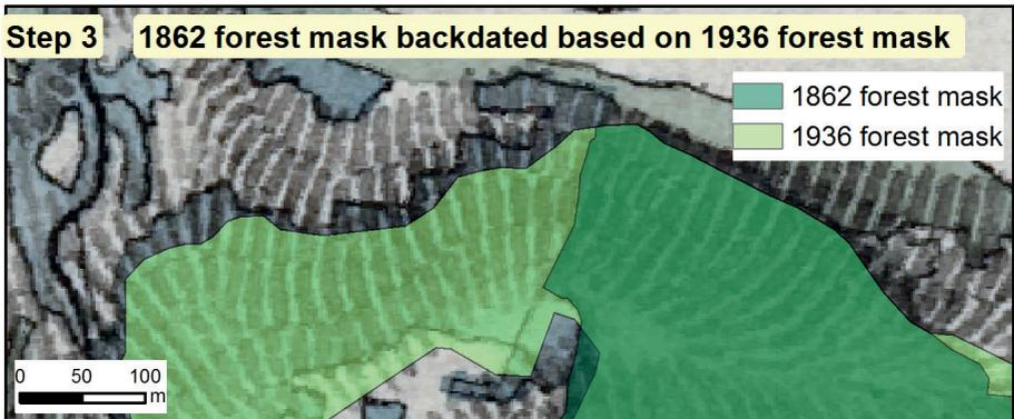
Fig. 2. Backdating approach used in the dependent vectorisation
