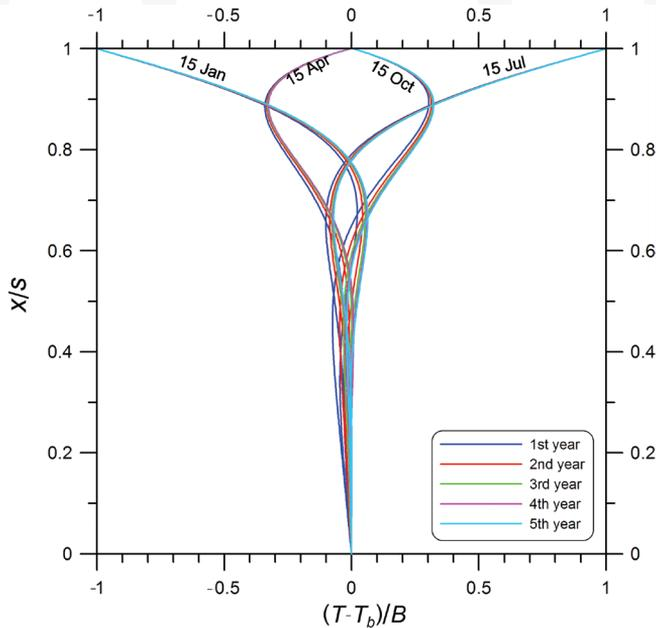
Fig. 2. Temperature profiles in the ground under natural conditions
