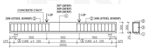
Fig. 1. Geometry and reinforcement of BFRP RC beams (dimensions in mm)
