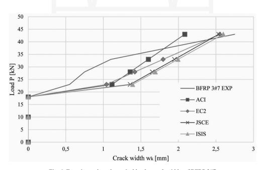
Fig. 4. Experimental vs. theoretical load – crack widths of BFRP 3#7
