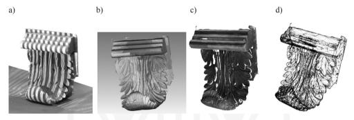
Fig. 3. Stages of the inventory of architectural details: a) the effect of the stripes on the object, b) point cloud, c) render, d) triangle mesh
