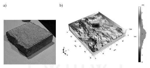
Fig. 4. a) a photography of a concrete sample testing, b) a graphical presentation of the surface obtained in the program MountainsMap
