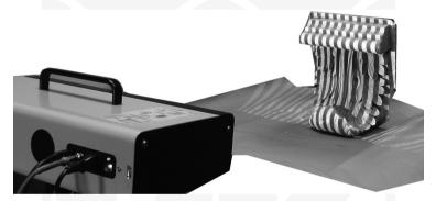
Fig. 1. Projection of stripes on the scanned object. Scanner: Smarttech Surface Scan3D
