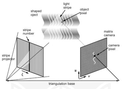
Fig. 2. The measuring principle based on the structured light [4]
