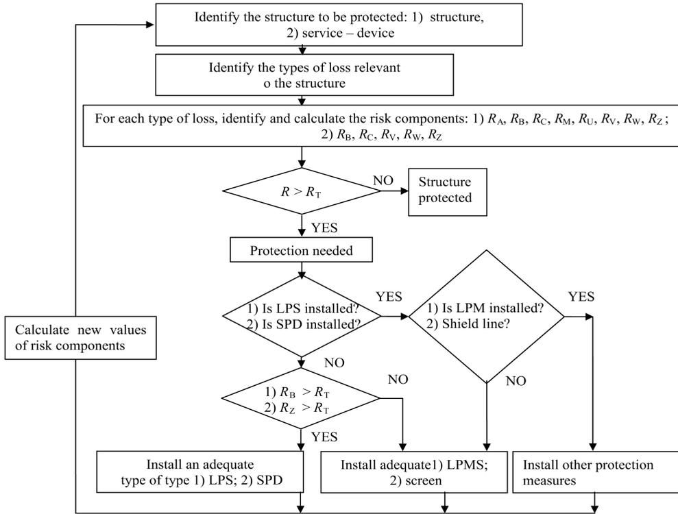
Fig. 1. The algorithm for deciding the need of protection and for selecting protection measures [1]
