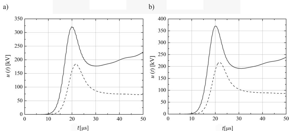
Fig. 5. Courses of surges for: a) trolley wires situated in the distance – 20 m from the channel of the stroke, b) the line NTL (for the distance – 40 m); the dashed lines – surges on both ends of the line, the solid lines – the nearest voltage to the stroke
