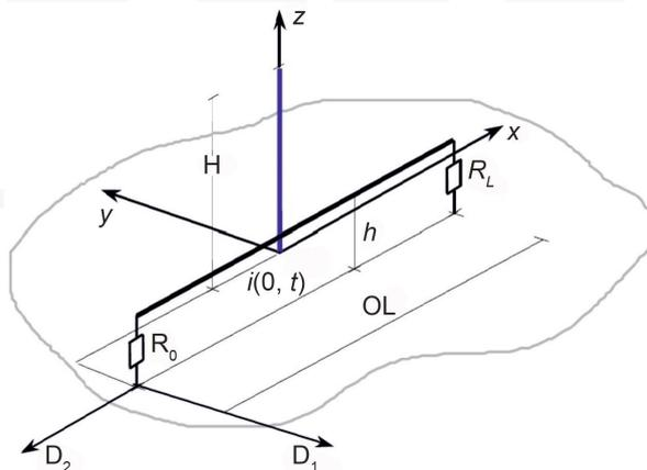
Fig. 4. The system of the discharge channel – transmission line [13]
