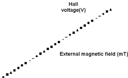
Fig. 3. Hall effect sensor characteristic
