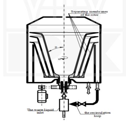
Fig. 1. The design concept of a centrifugal membrane device (CMD)
