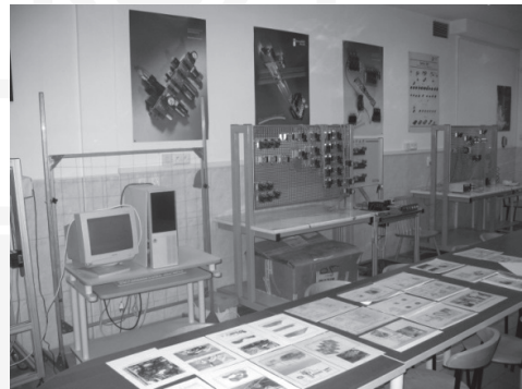
Fig. 2. Test rigs with the elements for pneumatic control systems
