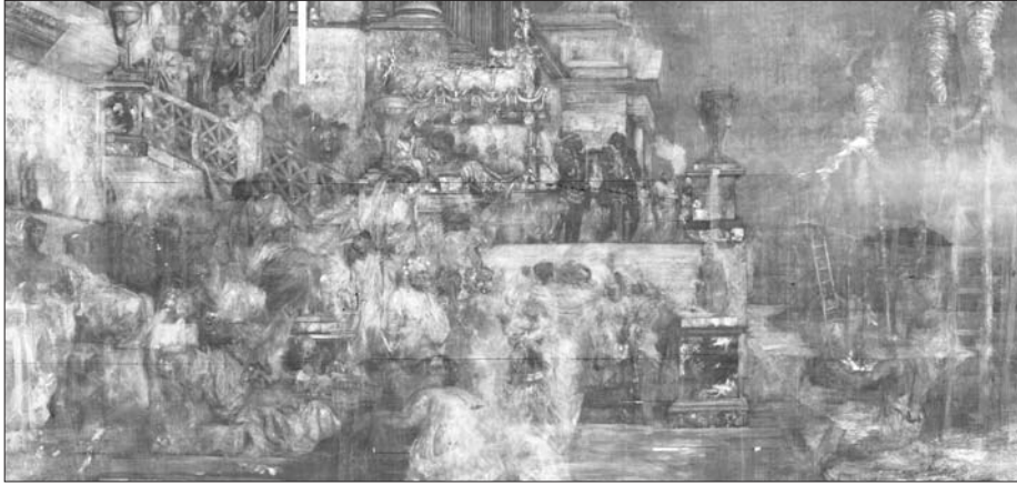
Fig. 3. H. Siemiradzki, Nero's Torches , 1876, National Museum in Kraków. X-ray image of the whole painting. The edges of the composition could not be analyzed because of a metal stretcher, which prevented the positioning of the detector. Photo by P. Frączek, M. Obarzanowski
