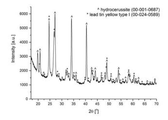
Fig. 6. Powder diffraction pattern of the yellow paint layer for the sample taken from the painting *Coronation of the Blessed Virgin Mary* from the cathedral in Oliwa
