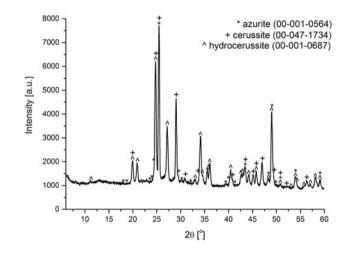
Fig. 2. Powder diffraction pattern of the blue paint layer for the sample taken from the painting *Servilius Appius*
