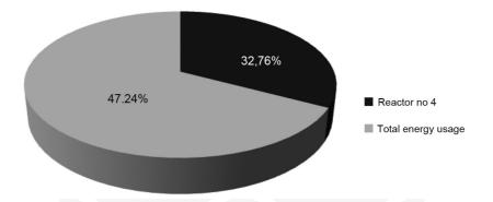
Fig. 6. Reactor no 4 average participation in total energy consumption during the analysed period
