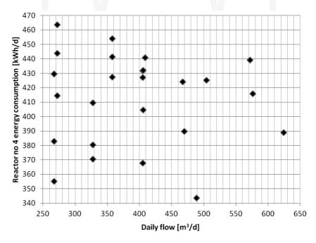
Fig. 4. Correlation of daily flow and reactor no 4 daily energy consumption
