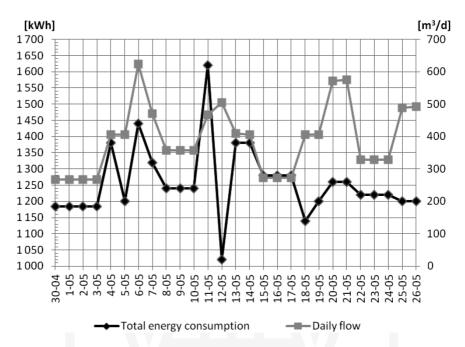
Fig. 1. Comparison of daily flow and plant's total daily energy consumption
