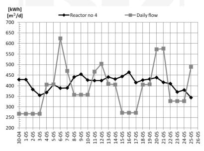
Fig. 3. Comparison of daily flow and reactor no 4 daily energy consumption
