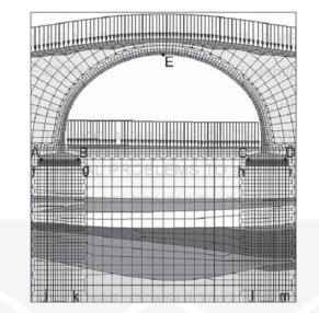
Fig. 5. Scheme of FEM mesh of the tunnel foundation on jet-grouting columns
