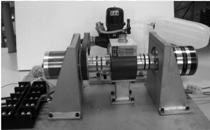
Fig. 2. Laboratory test stand of the hybrid drive
