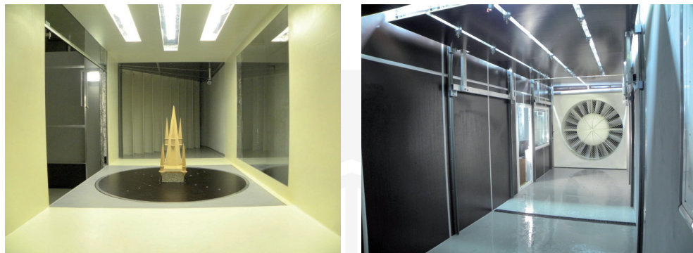
Fig. 3. Downwind view on aerodynamic section with historic tower model (left); View on the climatic chamber with 200 kW fan (right)
