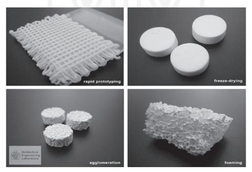
Fig. 4. Chitosan/TCP scaffolds prepared using varied techniques [33]
