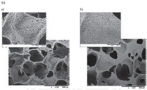
Fig. 3. The structure of scaffolds: (a): PUR + 20% calcite; (b): PUR + 40% calcite [11]
