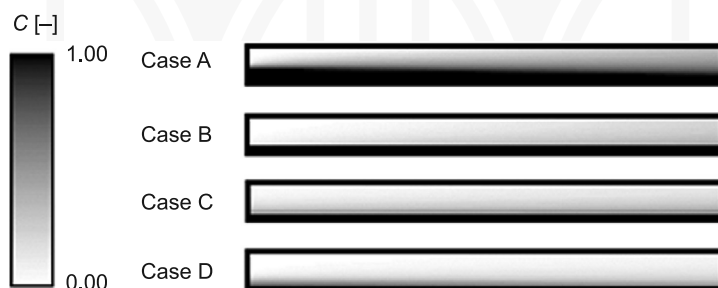
Fig. 2. Dimensionless concentration C of soybean oil in \text{scCO}_2 in the extraction module (solvent mass flow 0.5 g/min)
