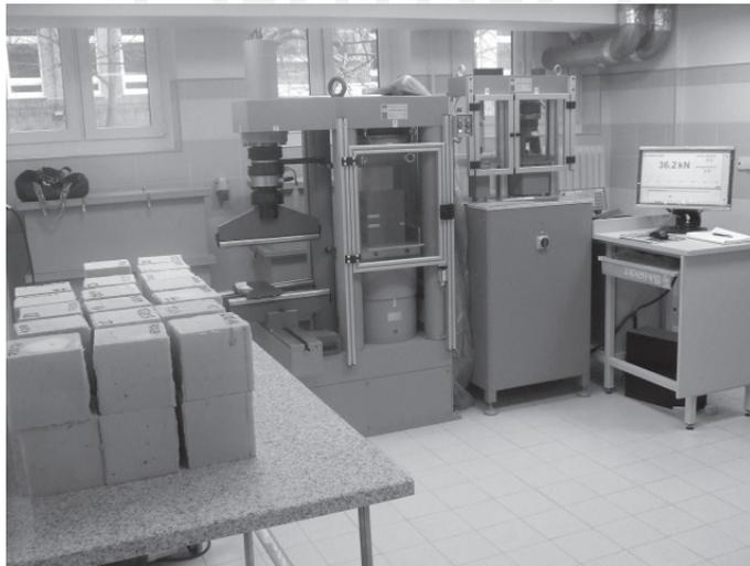
III. 3. Measurement of compressive strength
