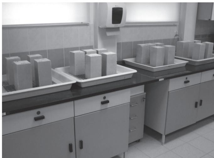
III. 1. Measurements of water sorption coefficients
